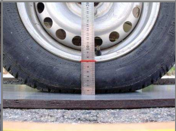
Obr. B31 – 130 kPa 750 kg
