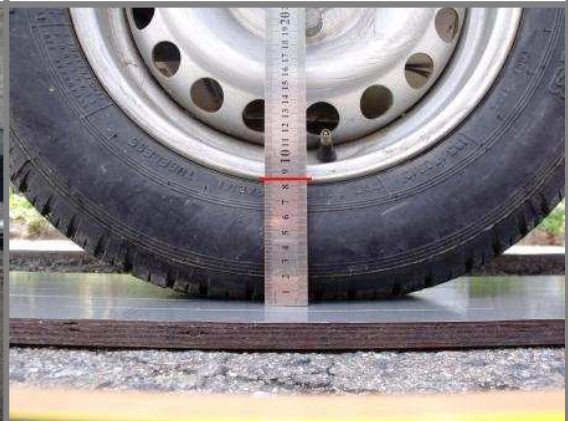
Obr. B15 – 330 kPa 750 kg
